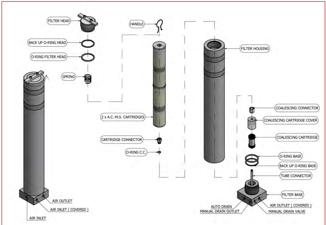
1. Unscrew the filter head counter clockwise.
