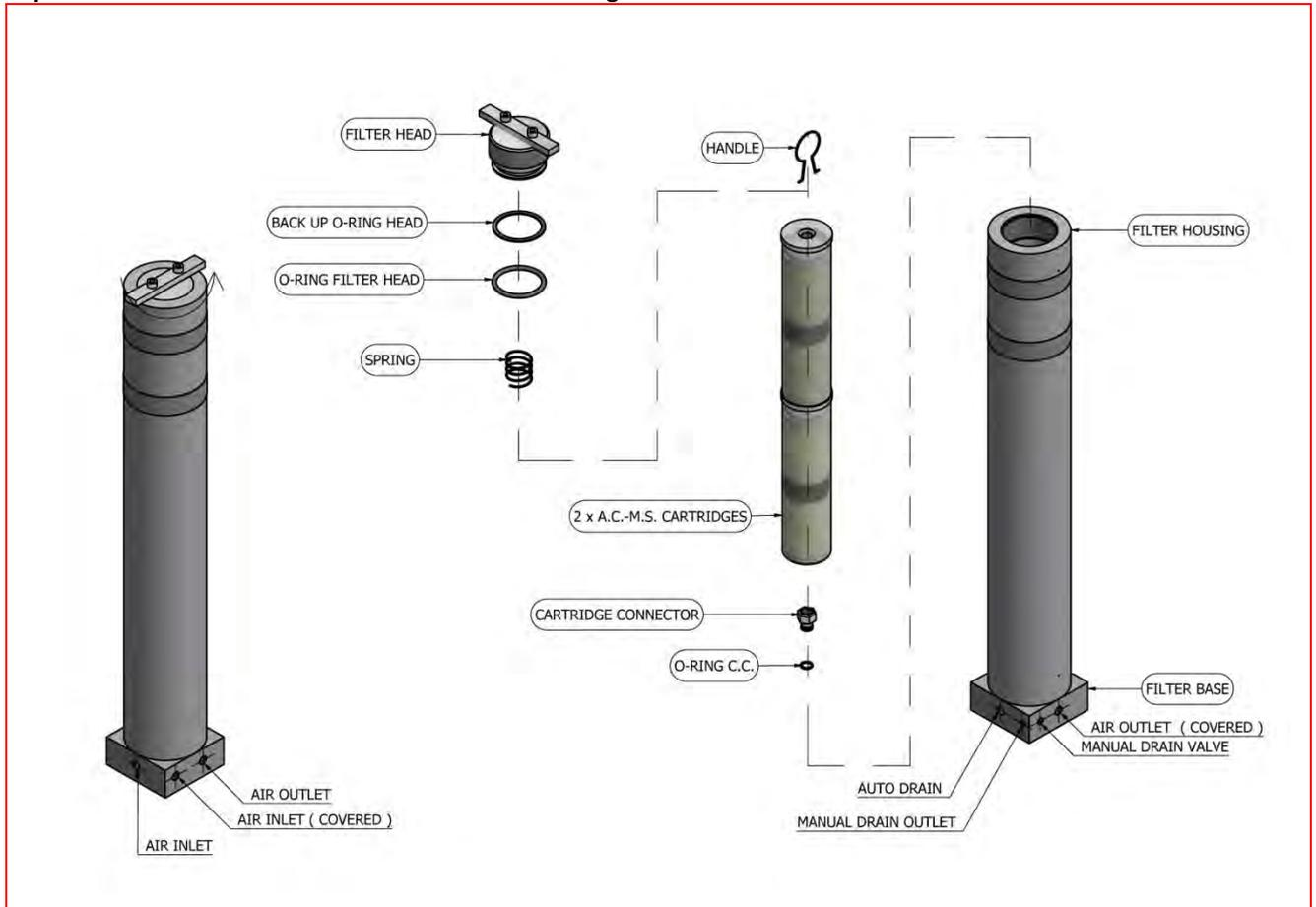
1. Unscrew the filter head counter clockwise.
