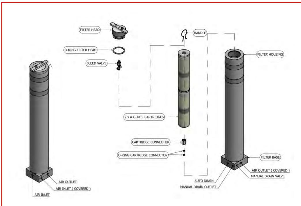
1. Unscrew the filter head counter clockwise.
