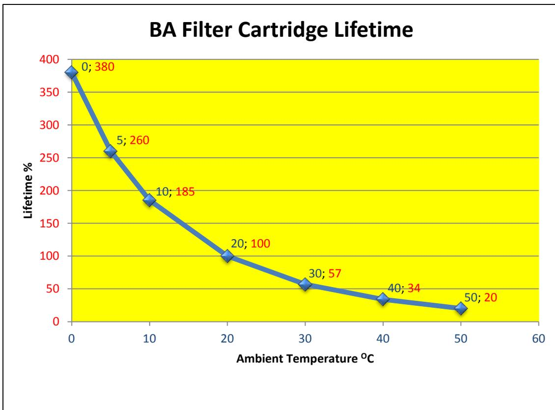
BA cartridge lifetime may change as humidity & temperature levels change. In summer a reduction in service hours is recommended, see above chart for examples relative to temperature.
