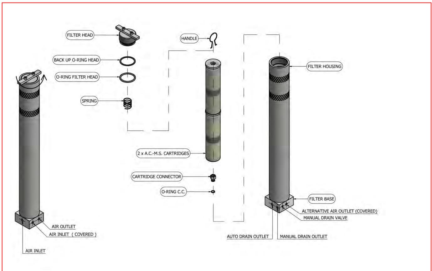
1. Unscrew the filter head counter clockwise.
