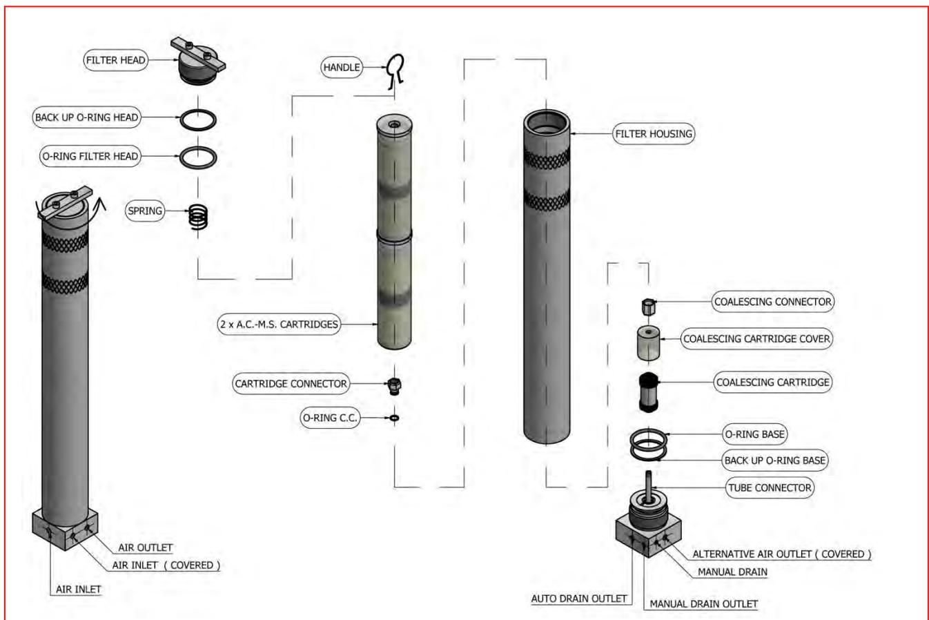
1. Unscrew the filter head counter clockwise.
