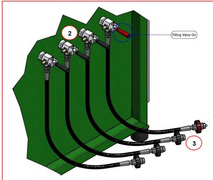
During the filling procedure, cylinder's temperature will rise. Let it cool down. Pressure will slightly drop. If you wish, re-connect the cylinder with the filling hose (following the same procedure) and fill until the maximum filling pressure.
