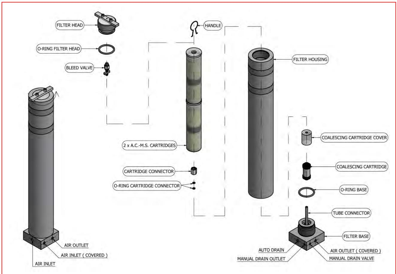
1. Unscrew the filter head counter clockwise.
